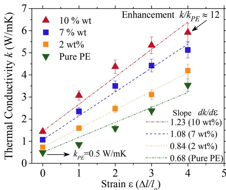
Figure. 3 Measured thermal conductivities of pure PE and PE-GnP composite as a function of applied strain. A highest  $k$  of 5.9 W/mK is achieved representing a 12-fold improvement over pristine PE. Increasing slopes of linear-fits point to the role of aligned GNPs in enhancing  $k$
