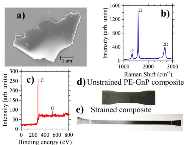
Figure 2 a) SEM image of a typical graphene nanoplatelet used in the study b) Raman and c) XPS analysis of GnPs. d) Unstrained and e) strained PE-GnP composite.
