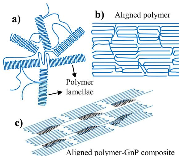
Figure. 1 a) Randomly oriented polymer lamellae in a semi-crystalline polymer b) Alignment induced by strain c) Aligned polymer-GnP composite.
