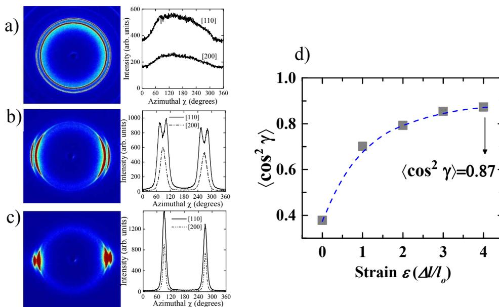
Figure. 6 a), b) and c) WAXS patterns for strains of 0, 2 and 4, in the pure PE sample d) Average orientation of PE chains in crystallites with respect to draw direction.
