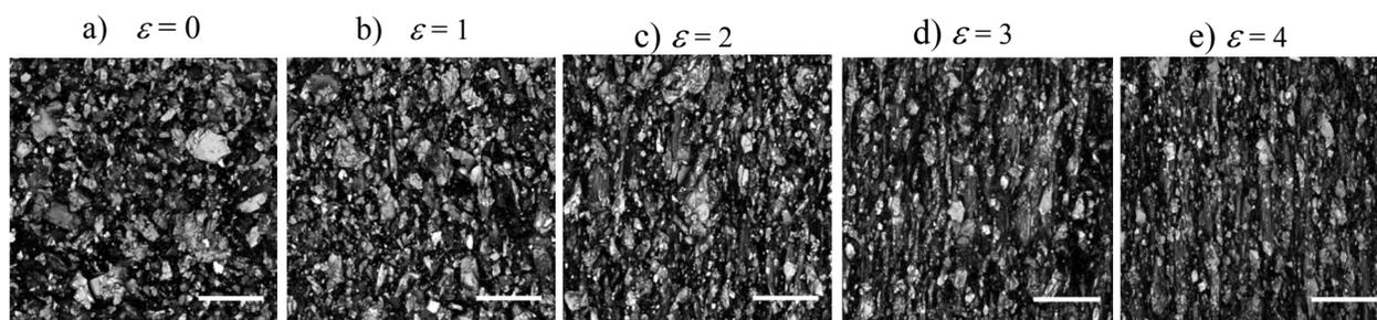
Figure. 4 Confocal microscopy images of GnPs in 7 wt% PE-GnP composite sample for different applied strains ( $\epsilon$ ) of a) 0, b) 1, c) 2, d) 3 and e) 4. Increasing alignment of GnPs with increasing strain is clearly visible in above maximum intensity projections. Scale bar = 20  $\mu\text{m}$ .
