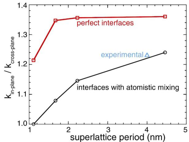
**Figure 4.** Anisotropy ratio of short period GaAs/AlAs superlattices. The ratio is lower when interfaces have atomic mixing and increases with increasing period.
