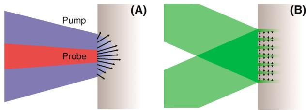
**Figure 1.** Schematic diagram of the laser excitation and subsequent heat diffusion pathways due to (A) the time-domain thermoreflectance (TDTR) setup and (B) the transient thermal grating (TTG) setup.
