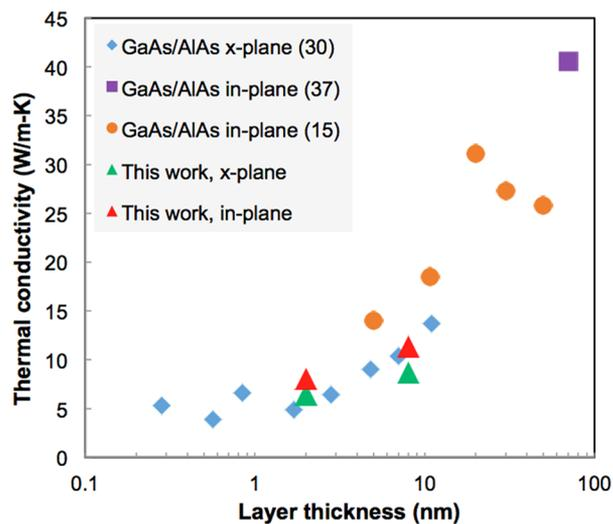
**Figure 3.** A comparison of the values of GaAs/AlAs thermal conductivities from the TDTR and TTG experiments with results from previous studies.
