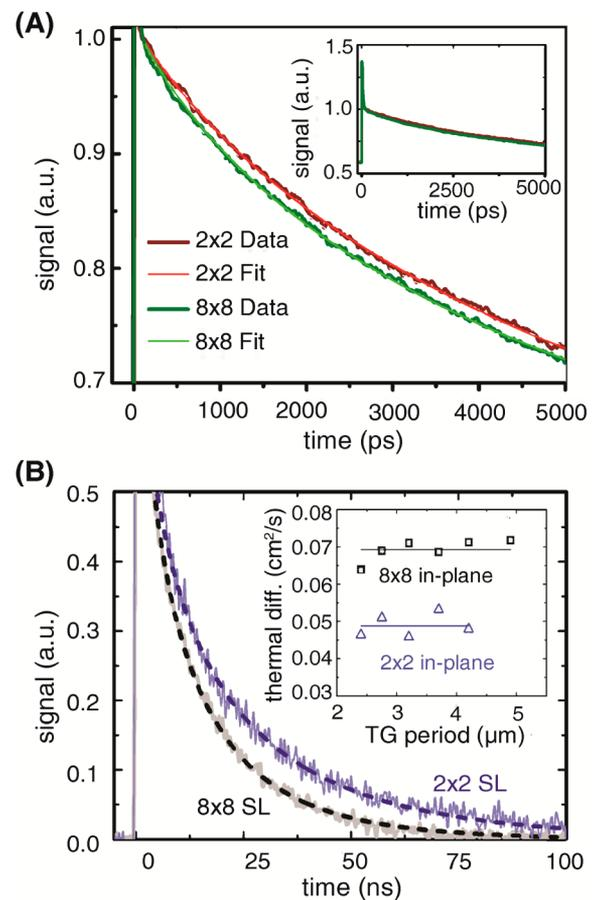
**Figure 2.** (A) TDTR and (B) TTG data and fits for the two SLs. The inset in B shows the thermal diffusivities of the two SLs at varying TG periods.
